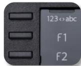
The 8018 DeskPhone uses 3 preprogrammed keys to access some features. In this case, the icon of the feature is printed on the paper. Use the feature by pressing the corresponding key. When activated, the LED corresponding to the key remains lit up. Press the corresponding key to deactivate it.
